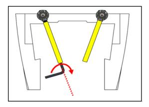
Before the set screws are fully tightened with the Allen key, the left-right balance of the product is adjusted.
