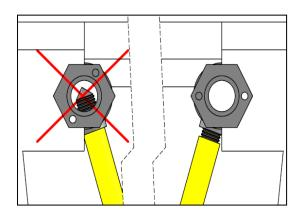
Check whether the fixing screw is zero to the inner surface of the mounting apparatus so that the screws on the wall can pass.
