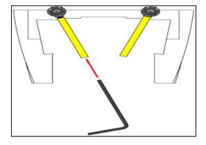
Adjust the left-right balance of the product before the set screws are fully tightened with the allen screw.
