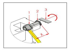
Fix the parts numbered 1 and 2 to the product with the tightening apparatus numbered 3. Measure X distance.
