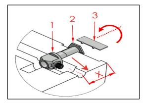
Measure X distance in the product, reduce 5.0 mm from the measured distance and adjust the stud length.
