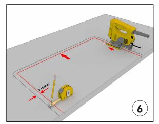
Cut by marking again from inside up to (X + 5 mm) of the mark.
