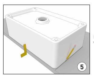
Place the product on the underside of the countertop on a line with the foreside. Mark the cutting location.
