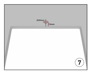
For armature hole position, mark the center of the reservoir and drill the hole from the marked part to the back side to 70 mm center with a 35 mm diameter punch.
