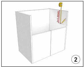
Mark the distance from the upper surface of the cabinet to the base of the sink as h+1.5 mm.
