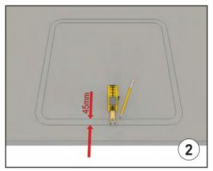
Remove the product. Mark the cutting line parallel to the 45 mm inner side of the marked line.
