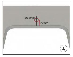
For armature hole position, mark the center of the reservoir and drill the hole from the marked part to the back side to 70 mm center with a 35 mm diameter punch.
