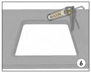
Apply silicone to the mounting surface of the countertop and to the cutting surface when using a wooden countertop.
