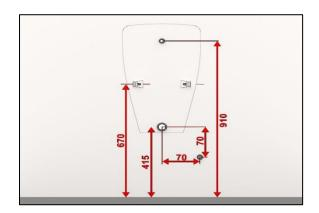
Prepare the infrastructure in specified sizes and align the water inlet and waste water outlet with the wall surface.
