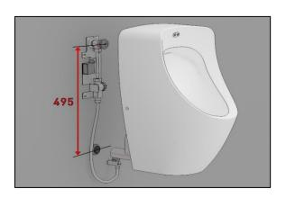
Fix the water inlet system of the urinal to the installation location in the specified sizes. Place the product temporarily on installation location.
