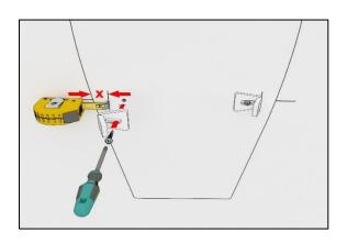
Fix the installation apparatus to the wall by leaving a space equal to the measured wall thickness.
