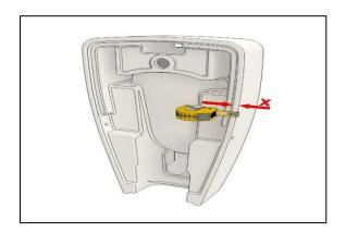
Measure the installation hole wall thickness of the product.
