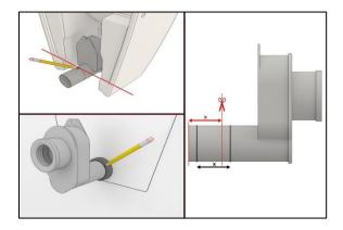
Adjust the drain pipe length as shown.
