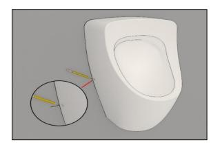
Draw the mounting hole axes and all base edges of the product on the wall.
