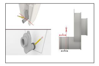
Adjust the drain pipe length as shown.
