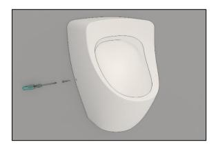
Complete the installation by fixing the screw heads on both sides.
