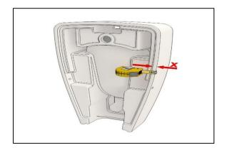
Remove the product and measure the installation hole wall thickness.
