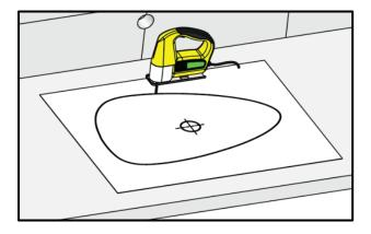
Attach the cutting template to the counter and cut the counter from the marked part.
