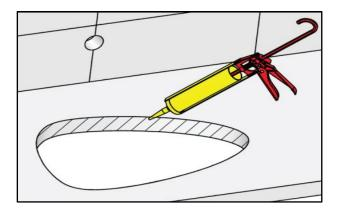
Apply silicone to prevent moisture in case of using wooden counter.
