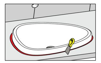
Remove excessive silicone and wait for 24 hours.
