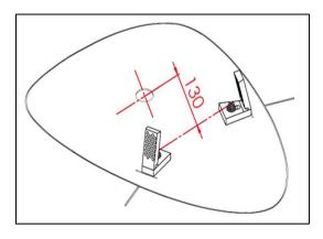
Make sure that the waste water outlet is located on the wide base side of the washbasin.
