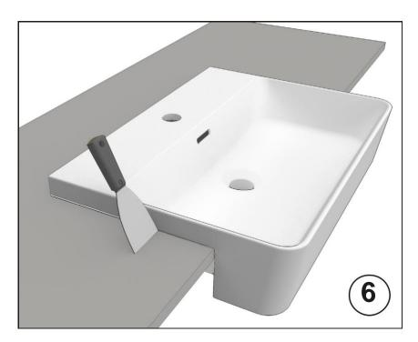
Excess of the silicone overflowing from the edges is taken to have a smooth surface.
