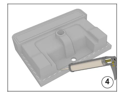
Silicone is applied to the surface where the washbasin will be installed.
