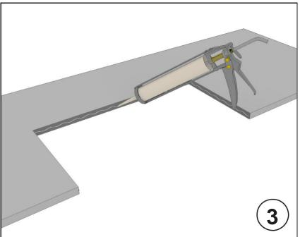
In case a wooden countertop is used, silicon is applied to the cutout place to prevent contact with moisture.
