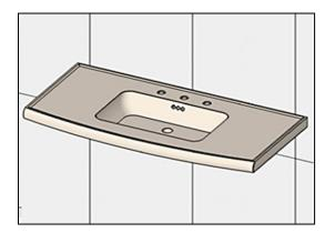
Install the washbasin and do not tighten nuts completely.
