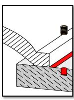
Open dowel holes and insert dowels. When using wooden countertops, fixing should be done with wood screws.
