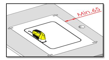
Attach the cutting template to the counter and cut the counter from the marked part.
