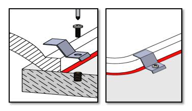
Fix the washbasin. When using wooden countertops, fixing should be done with wood screws.
