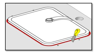
Place the washbasin and remove excessive silicone.
