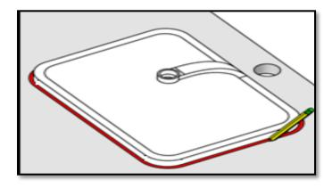
Place the washbasin under the counter temporarily and mark the edges.
