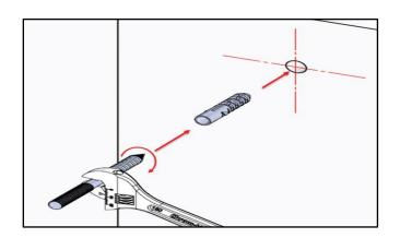
Insert dowels and studs into the holes.
