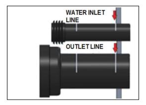
Fix the drain pipes to the installation and mark the areas shown with arrow.
