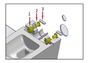
Fix the parts numbered 1 and 2 to the product with the tightening apparatus numbered 3.
