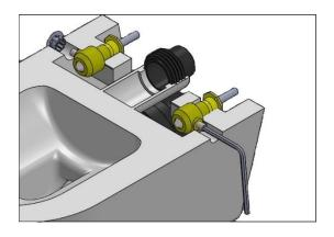
Place the product and complete the installation by inserting the allen screw to the set screw from side installation holes.
