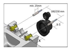
Measure **X** distance in the product, reduce **5.0 mm** from the measured distance, adjust the sleeve-headed stud lengths and turn the sleeve-head holes sideways.
