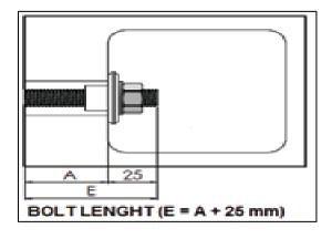
Adjust the bolt length wall thickness of the installation system by leaving a +25 mm margin.
