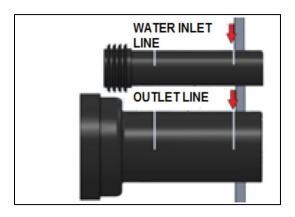
Fix the drain pipes to the installation and mark the areas shown with arrow.
