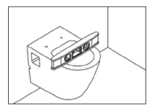
Place the toilet and adjust the balance before the studs are fully tightened.
