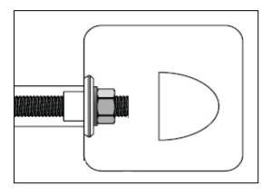
Tighten the studs and attach the stud caps.
