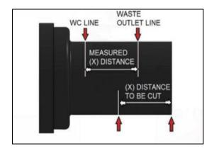
Shorten the waste water drain pipe as the distance between two marks.
