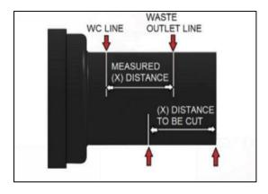
Shorten the waste water drain pipe as the distance between two marks.
