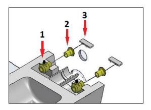
Fix the parts numbered 1 and 2 to the product with the tightening apparatus numbered 3.
