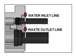
Fix the drain pipes to the product and mark the areas shown with arrow.
