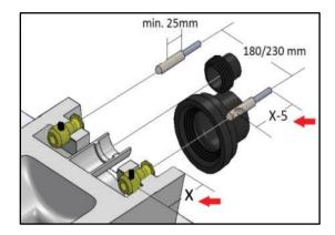
Measure **X** distance in the product, reduce **5.0 mm** from the measured distance, adjust the sleeve-headed stud lengths and turn the sleeve-head holes upwards.
