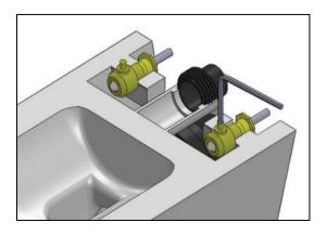
Place the product and complete the installation by inserting the allen screw into the set screw from the cover installation holes.
